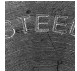
BF + DF Incident and grazing lighting
