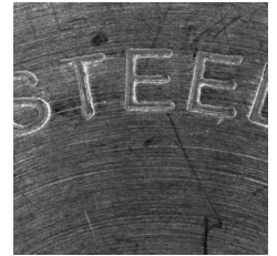
BF + DF Incident and grazing lighting
