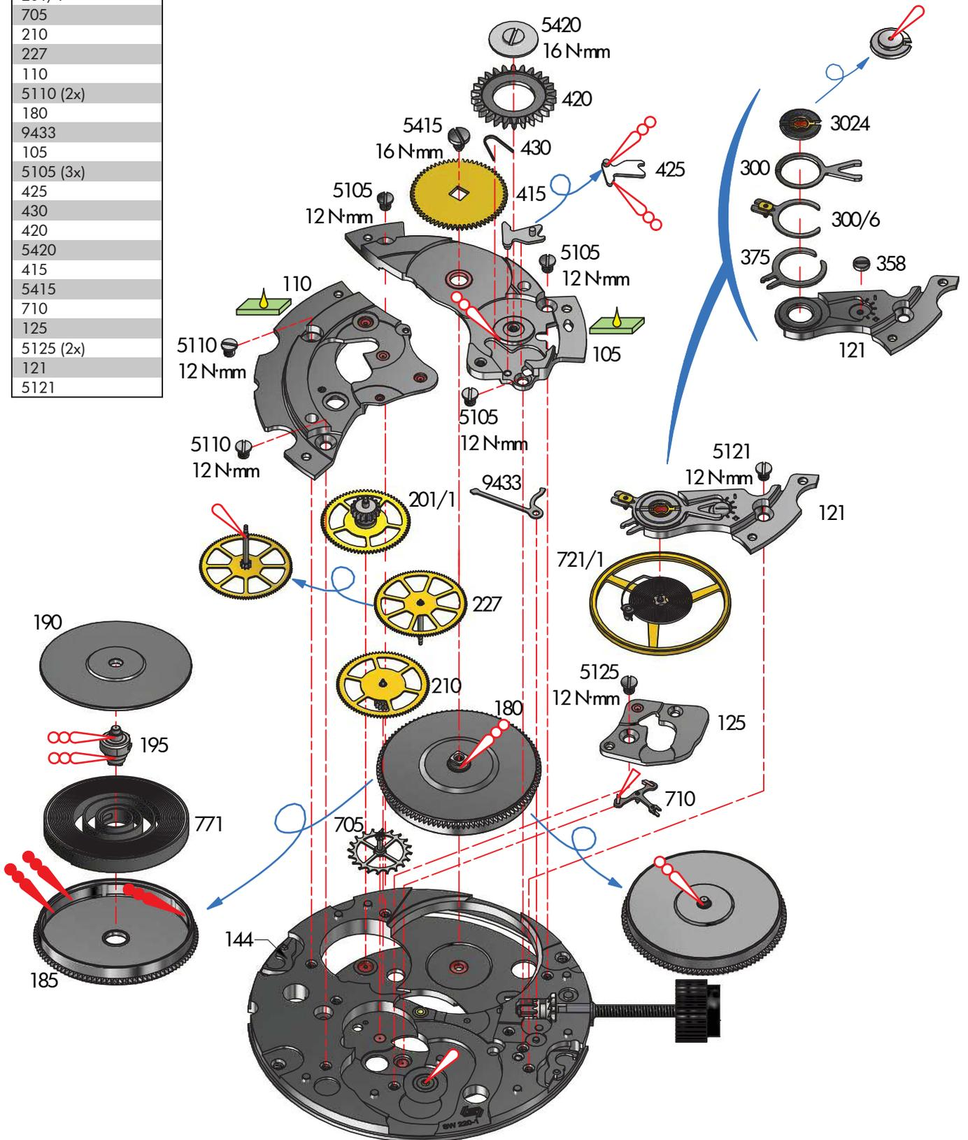
Mécanisme automatique - Automatik- Mechanismus - Self-winding mechanisms
