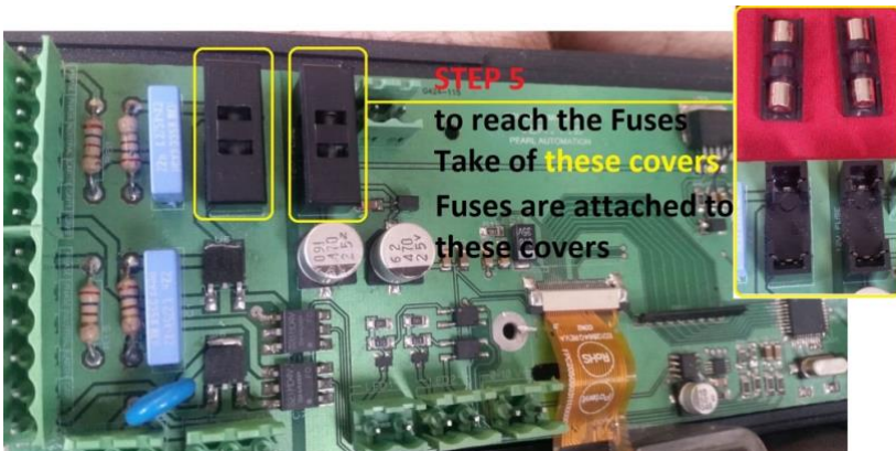
Step 5 To reach the fuses, take off these covers. Fuses are attached to these covers.
