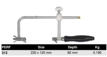
Saw frame with wooden handle, screws and fixing plates to hold the saw blades. Equipped with a wing screw to adjust the tension of the saw blades.
