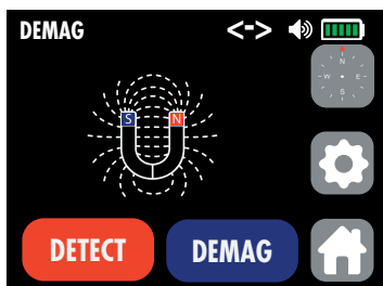
Display of the submenu DEMAG in demagnetization mode (beeps are heard during the cycle. We will also see that the S and N poles flash and cross each other throughout the cycle)
